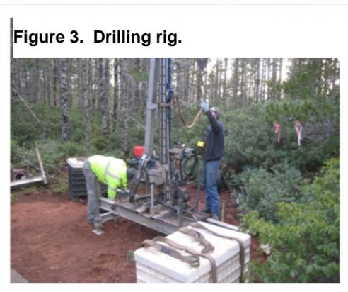
A low impact, light drilling rig (Figure 3) would be moved to each site by truck and lifted by boom onto a temporary 4-foot by 11-foot raised metal platform. Prior to beginning drilling at the next location, sealing of the hole, spreading of drill cuttings to blend with the natural slope, and removal of all equipment and materials would occur.
